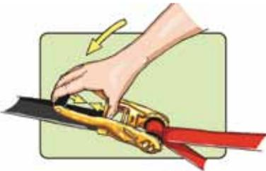
8. In order to secure the ratchet push the metal square up again and close the ratchet fully. To do so push lever down towards the webbing loop. For double security use the remaining line and tie the ratchet lever together with the line. This will prevent an accidentally opening of the ratchet.
