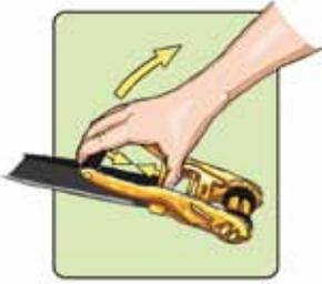
4. To open the ratchet and push the inner square up with your thumb towards the handle (the locking mechanism will release) as shown on picture. Now you can move the ratchet lever towards yourself.
