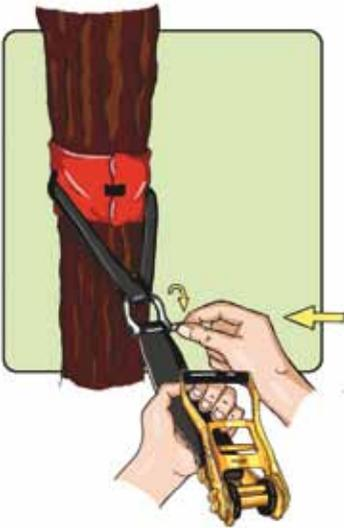
3. Repeat the same as you have just done on the other side. First wrap the tree protector around the tree, attach tree/anchor slings using velcro fastener. Now take the ratchet and link to sling using the second stainless steel bow shackle. Tip: Leaving the bolt slightly loose (tight minus a quarter turn) makes it easier to undo later. Make sure the webbing loop of the ratchet is placed on top of the shackle bolt. The lever of the ratchet should face up for easy tightening.
