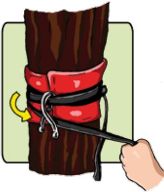
5. Within the last last layer pull the strap underneath the shackle back to the loop. Always try to keep the strap tight.
